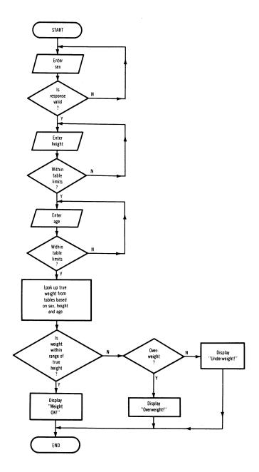
Fig. 4-1. Weight example program flowchart.
