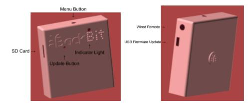
The **Menu Button** up top allows you to return to the menu once a program is running. The **Indicator Light** lets you know when requests are being made to the cartridge. The **Micro-SD Card** slot accepts any microSD card formatted to FAT32 or FAT16. The slot is designed so that cards will not "fall in" to the cartridge and will be easy to remove.
