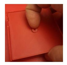
1. Use fingernail to remove peg from the back of the cartridge. Don't lose it!
