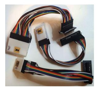
The <u>**Clip Adapter**</u> (one included with tester, additional clips available for purchase) provides a convenient way to attach a chip clip for in-circuit testing. You will need both a clip adapter and jumper extension wire for each chip clip you want to use.
