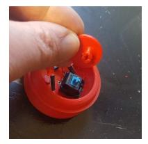
2. Apply key cap on the blue switch. Wiggle and push until it sets.
