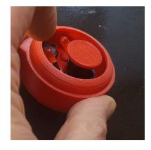
3. Push the LEDs down or to the side slightly so that they aren't touching the key cap.
