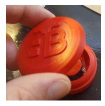
6. Center the lid on the button so that the antennae in the logo line up with the flat side of the button.
