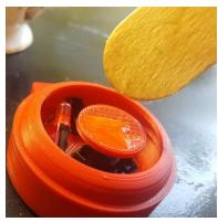
5. Dip a wooden stick into the acetone, and apply a few drops to the top of the key cap until there is a thin layer on top (but don't let it overflow).
