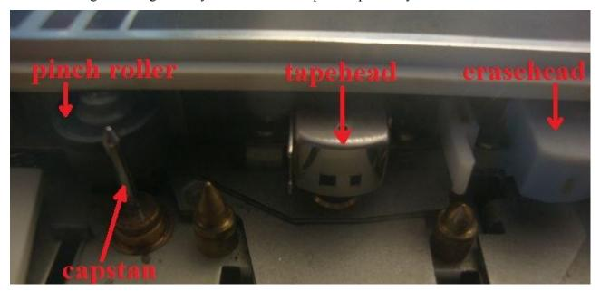
So in other words... always make sure that your datasette (or other kind of tape recorder) is in perfect working condition. A backup or restored tape is only as good as the recorder is was made on. If you use a crappy recorder, you'd get crappy recordings!
