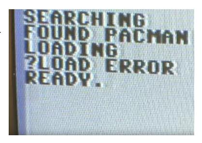
datasette (and any other kind of tape drive used for home computing in the 80's) is tapehead alignment, also referred to as azimuth. Make sure that your tapeheads are aligned properly.
