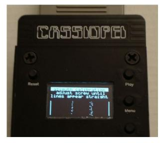
Switch off your CBM computer, connect the datasette to your Cassiopei, press the play, wind or rewind button and switch on the CBM computer. The Cassiopei will detect the datasette (because the sense line is active caused by the pressed play, wind or rewind button) and will show a different screen. This is the .TAP creator mode (a.k.a. the backup/restore mode).
