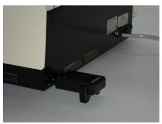
As the image above demonstrates, the PET/CBM 2000 and 3000 series require the use of an additional stand. You can attach this by removing the back cover of the Cassiopei and then slide the stand gently over the cassetteport connector, then replace the back cover.
