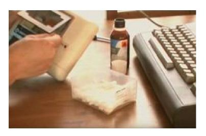
Don't forget to clean the erasehead too, although you don't need it for reading back tapes it is very important for writing. When cleaning of both heads is done, make sure to let it dry for 15 minutes before using it, you don't want your tapes to get wet OR to stick to your wet tape head while playing.
