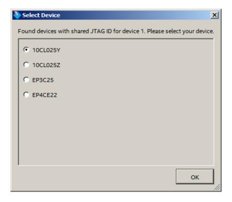
Now either click on the picture of the EP3C25 and click the Change File button, or double-click the "<none>" in the File column of the EP3C25's line in the top panel.
