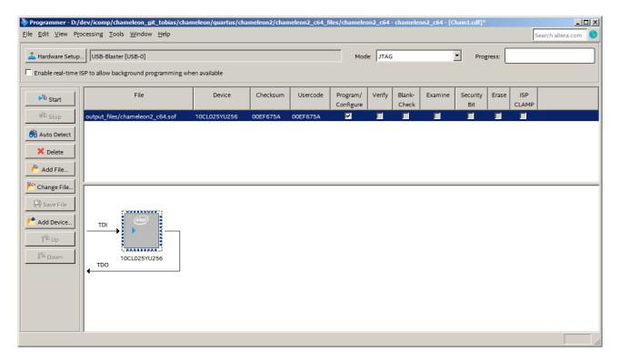
Finally, click Start, and the project should be uploaded to the FPGA.
