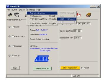
Now load the micro-controller hex file by clicking on file->Load hex file. The final step is to click on the "Run" button within FLIP (at the bottom left of the window) and watch the program do its magic. After programming the micro controller, FLIP will indicate the successful steps with a green light next to the action tags:
