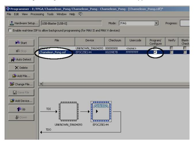
When using Chameleon v2 Hardware either click on the picture of the 10CL025V and click the Change File button, or double-click the "<none>" in the File column of the 10CL025V's line in the top panel.
