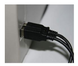
In stand-alone mode, you will need at least the breakout cable to connect to Chameleon, because it will provide power to the cartridge. With the second version of the Chameleon, please use the mini USB connector at the bottom/left for power:
