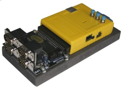
Connect the breakout cable and supply power to the whole setup through the USB connector of the breakout cable (first version of the chameleon) or the mini USB connector at the bottom/left (second version of the chameleon). Make sure that your power supply is strong enough! With the docking station, we recommend to use a 5V/1000mA power supply. If available, use a 5.2V/1000mA power supply, but **never** use any higher voltage than 5.2V. Only use regulated power supplies.
