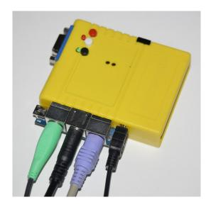
Make sure that the power supply can deliver at least the 2.5W (5V and 500mA) that's specified for a USB connection. The Chameleon hardware will take about 2 Watts of power, so make sure that your keyboard and mouse don't overload the power supply! Most PCs don't have any trouble supplying Chameleon with power. Note that some PCs don't provide power without a data connection on a USB port. In that case, please use a separate power supply.
