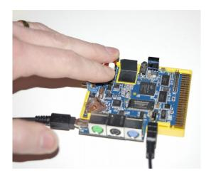
Then release the right (reset) button, but keep on holding the left button. As the last step, release the left button:
