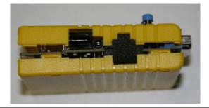
Remove the bottom by tilting it away; the left side (weakest side of the top) will now come off fairly easy, almost no force is required. Remove the foam from the case and keep it in a safe place. The foam on your cartridge may look different.
