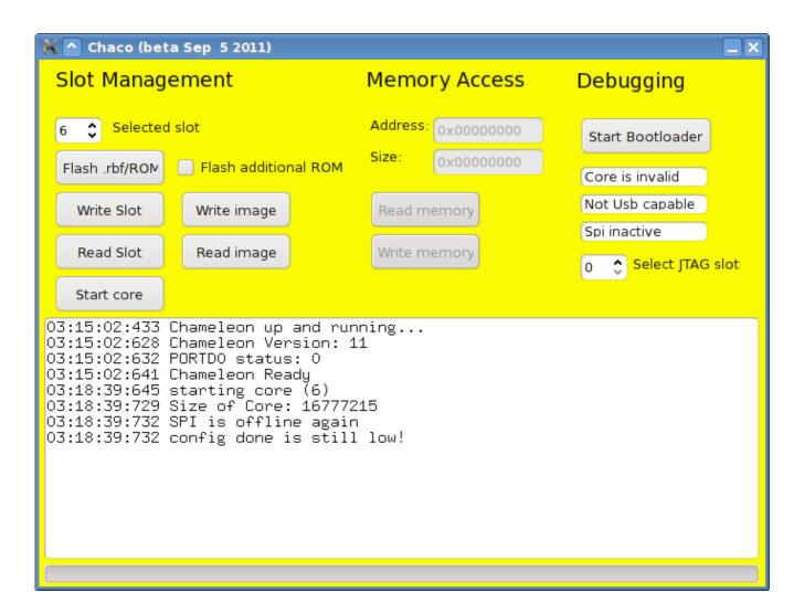
The error message in the window reflects what you should see on Chameleon: The red LED should blink seven times, then pause, then start over with blinking.
