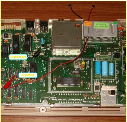
The Mini-Clip Connections for a C64 (or 64C) can be done in Just Minutes. (Easily connect the HIRAM and CAEC wires to any version of the 64) For 64C, the HIRAM wire connects to Pin-28 of the MPU (processor) and the CAEC wire connects to Pin-5.
