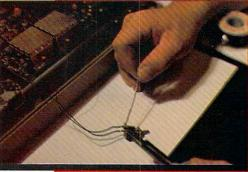
FIG. Soldering ends of hookup wire onto two switch terminals.
