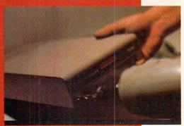
Drilling a 3/16" hole in the plastic top cover of drive case.
