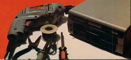
Tools/parts needed: electric drill and bit, wire cutters/pliers, rosin-core solder, soldering iron, hookup wire, Phillips screwdriver, 1541 drive.
