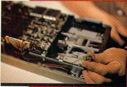
FIG. The completed solder connec-8 tions to jumper and switch.
