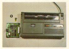
The Okimate 10 Color Printer, side by side with its attendant **0** user-replaceable thermal print head and **2** Plug 'n Print module. READER SERVICE NO. 268
