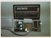
Inside Xetec GPI: **0** 4K interface ROM; **2** 2K RAM buffer; **3** 6802 microprocessor; **3** interface clock crystal; **5** setup switches
