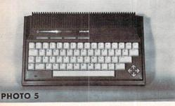
The Plus/4 keyboard has relocated the function keys to the top row and grouped the cursor keys into a diamond pattern.
