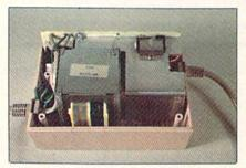
Power supply: transformer (left), rectifier, and voltage regulator boards.
