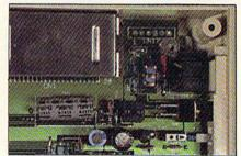
Clockwise from top: cart port, power connector, on/off switch, reset button.
