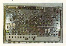
The upper radiation shield of the C-128 serves as a heat sink as well.
