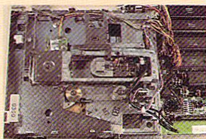
Closeup of drive mechanism, which incorporates a brushless DC motor.
