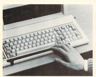
The 10' grounding cord of the Model 9250 is fastened to a 3.5' right angle strip extension that folds down and underneath the keyboard. The cord's opposite end should be fastened to a suitable ground. READER SERVICE NO. 200
