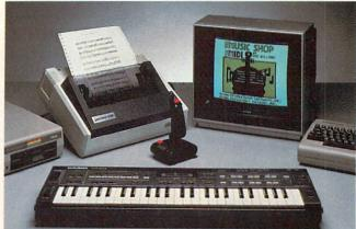
Useful, or necessary, for operation of The **Music Shop** for MIDI: 64, monitor, printer, drive, joystick, keyboard. Not shown: MIDI Interface Card. READER SERVICE NO. 280
