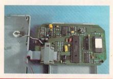
Interior views of Magic Voice (left) and Voice Command Module. Note the two kilobytes of ROM and the onboard microprocessor in the latter.
