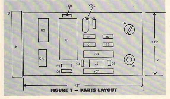
A standard piece of perforated 100th inch center board was used for circuit board. Layout and wiring techniques are not critical. Wire wrap sockets were used (the fastest way to get the circuit running).
