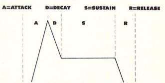
Figure 1: Illustration of an ADSR envelope.
