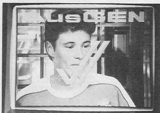
Example overlay. The border, "AusGEN" and Amiga checkmark are coming from the Amiga and are overlaid on the video.
