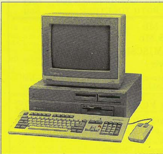
A2000 with dual 3.5" drives & 1 x 5.25" drive
