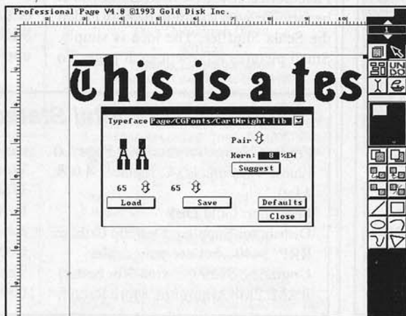
The new Kerning control requester allows individual letter pairs to be adjusted and the settings for an entire font saved
