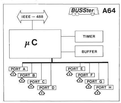
IEEE-488 64 DIGITAL CHANNEL DATA ACQUISITION INPUT MODULE
