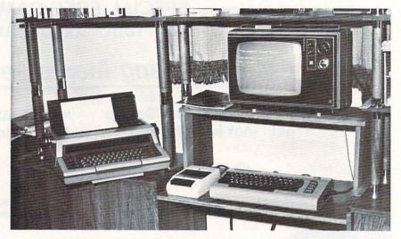
The SCM Typetronic fits in well with my C-64, Datasette and TV monitor. The Cord interface is not visible in this picture, but sits directly behind the Typetronic.
