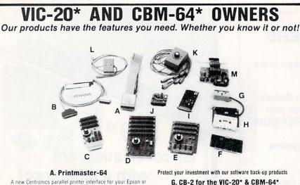
A new Centronics parallel printer interface for your Epson or Gemini printer that prints the "full" Commodore graphics set or ASCII data. This "cartridge" adds 16 new commands to the C-64\* for simplified printer control.
