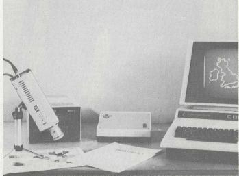
The MicroSight package: CCTV camera and MicroEye interface
