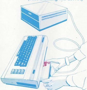
The IEEE 488 is probably the most powerful and flexible of all interfaces and at DAMS we have now harnessed it into a special cartridge, which plugs easily into the back of your VIC 20 or Commodore 64 computer, allowing for the connection of all peripherals previously associated with the PET range to the VIC!
