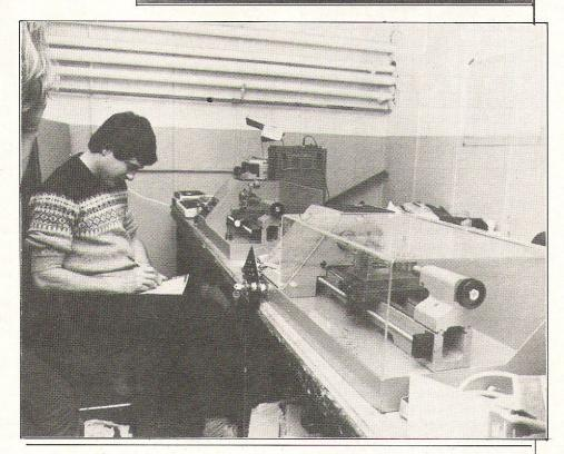
Colne Robotics' latest venture is a lathe. Once again it's designed especially for educational purposes. It can teach newcomers to the lathe how any lathe works but especially how a computerised lathe works. The piece to be turned can first of all be designed on the monitor and can be viewed as a three dimensional object. It is therefore possible to see exactly what the finished piece will look like before work starts.
