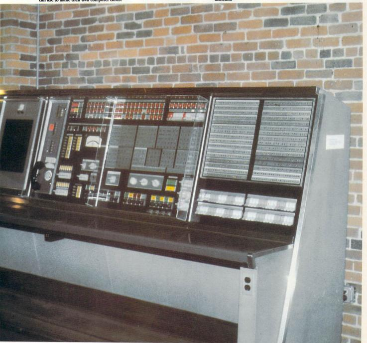
Main control panel of the AN/FSQ-7, the 1950's US Air Force computer for the radar early warning system (SAGE).
