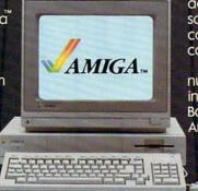
advantage of the custom chips and the software support routines in the writable control store on the Kickstart™ disk that comes with every Amiga computer.
