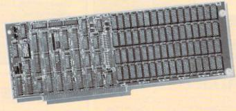
Micron Technology has announced a 2 megabyte board for the Amiga 500, 1000 and 2000 series. The memory board is inserted into an expansion slot on the motherboard of the Amiga 2000, while an expansion chassis must be purchased along with the memory board for the 500 and 1000.
