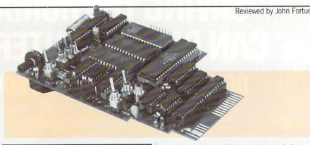
At 4 MHz, the Turbo Processor can run programs four times what they run at in the 64.
