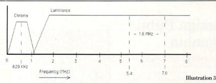
minance signals in an unencoded state. Connected to another SVHS deck, the S terminal lets you copy a tape while bypassing the encoding/decoding process that degrades the video signal. Connected to an S-compatible monitor you get a display that is sharper, with colors that are cleaner than any standard video monitor short of RGB.
