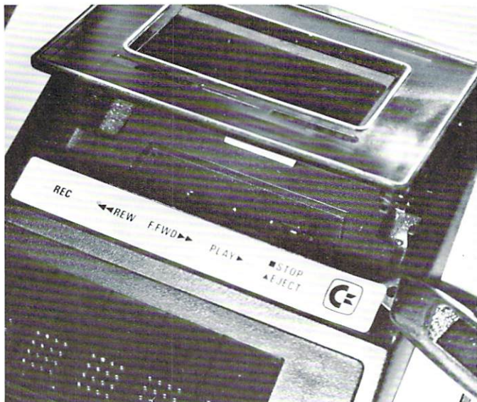
Figure 2 - To get at the screw hole in the push-button-eject model you must remove the metal label strip as shown.
