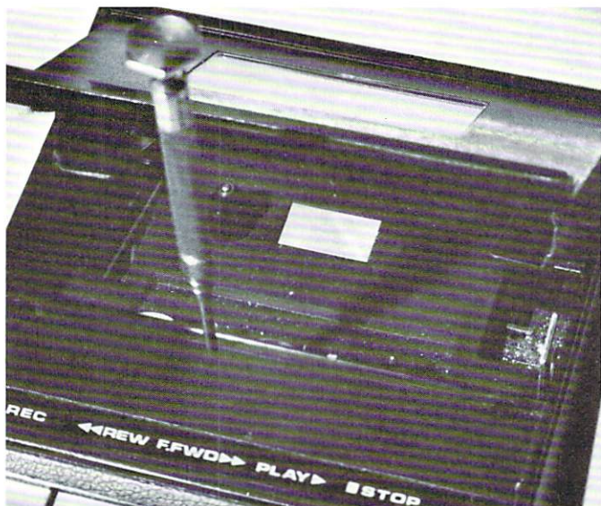
Figure 1 - Location of the adjustment screw hole for the hand-lifted cover model.
