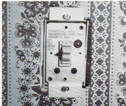
Photo 2: The wall switch module replaces the standard wall light switch. As with all the remote modules, it can be locally activated without the command console.
