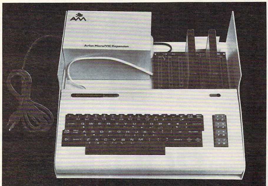
Arfon Micro VIC-20 Expansion Chassis shown here with cover removed.
