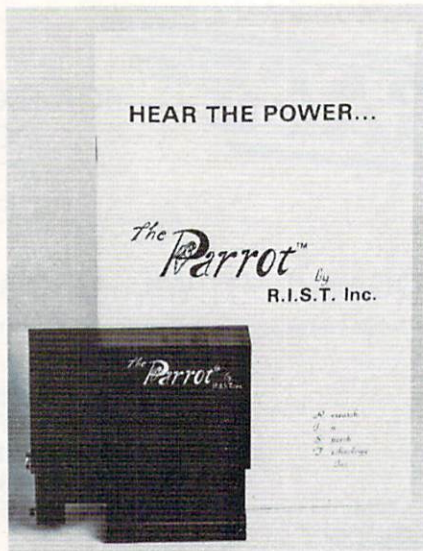
The Parrot is a 3" by 3" by 1 1/2" speech module for Timex/Sinclair computers.
