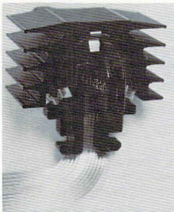
A print head from a dot-matrix printer. The ends of the tiny wires which form the characters are barely visible at the front-center of the print-head.
