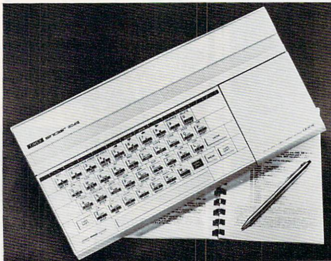
The Timex/Sinclair 2048 with 48K RAM and hidden cartridge slot (beneath cover at right).
