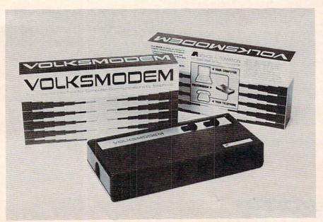
Anchor Automation's Volksmodem can interface with most personal computers via a separate cable. It is a direct-connect modem.
