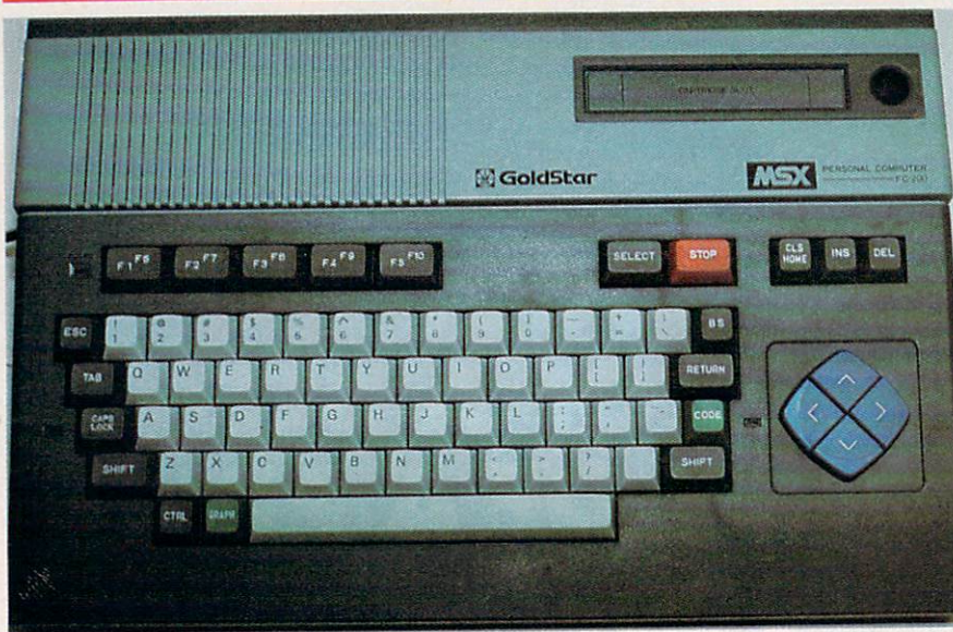
The GoldStar FC-200 MSX Personal Computer, a Korean creation. The keyboard layout is very similar on all MSX computers. Notice the editing keys, cursor keypad, and preprogrammed special function keys. The hatch at the upper right conceals the ROM cartridge slot. The hole next to it is a light pen holder.
