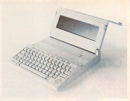
Commodore LCD: a second-generation lap portable with  $80 \times 16$  flip-up display, 32K RAM, internal modem, and eight built-in programs for under \$600.
