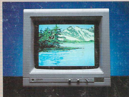
MODEL 220 14" Composite Color Monitor with Audio. Standard NTSC composite video signal input. Chrominance and luminance inputs available for Commodore, Atari, and other computers. Extremely low geometric distortion. Switchable to green or amber display. Built-in 2 watt audio. Optional: Tilt/Swivel Base available (Model 110-12)
