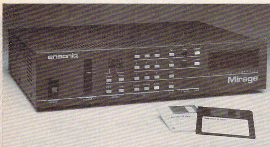
MIDI-controlled musical devices, like this $1,395 digital sampling instrument from Ensoniq with a built-in 3½-inch disk drive, are bringing computers and electronic instruments closer together.
