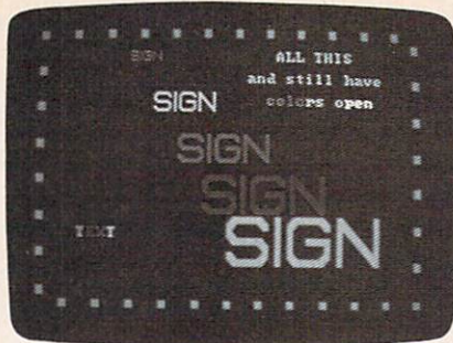
The IBM PCjr's PALETTE USING statement simplifies color control for graphic displays.
