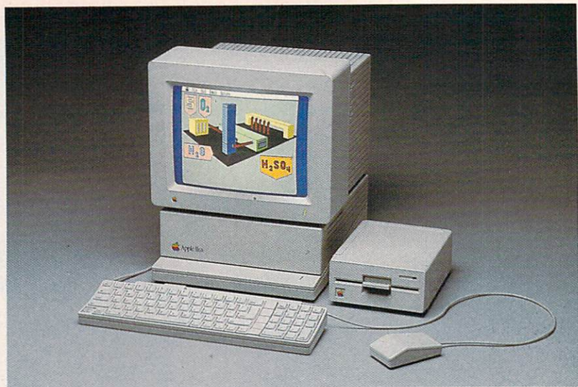
The Apple IIGS computer, shown here with the AppleColor RGB monitor and 5 1/4-inch drive, features 256K of RAM, high-resolution graphics, high-quality sound synthesis capabilities, and complete compatibility with existing Apple II software.
