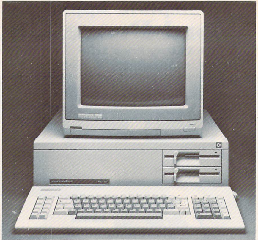
Commodore's $1,199 PC10-2 is a PC compatible with two disk drives, 640K of RAM, and five expansion slots. Commodore also introduced to the U.S. market the one-drive PC10-1 with 512K of memory.
