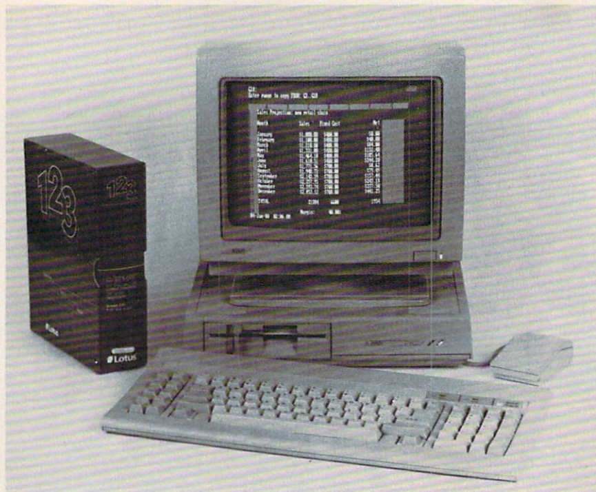
The Atari PC is a low-priced IBM compatible with 512K RAM and a wide variety of built-in display adapters and interfaces. Two models are priced at $499 and $699.
