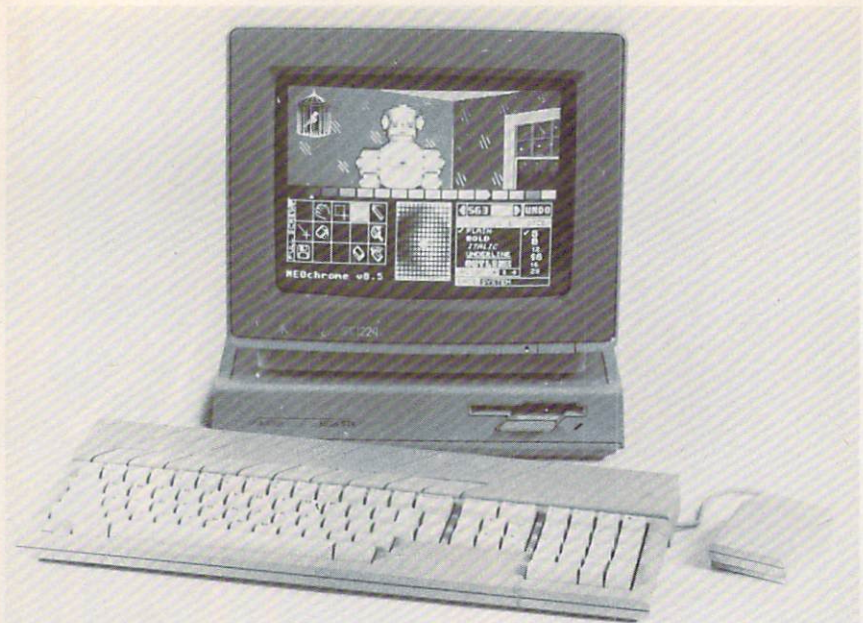
Atari's Mega ST is available in one-, two-, and four-megabyte models. All have a detached keyboard, internal floppy disk drive, blitter chip, battery-backup clock, and expansion bus.
