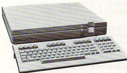
The Commodore 128D features a detachable keyboard and an internal 1571 5¼-inch disk drive.
