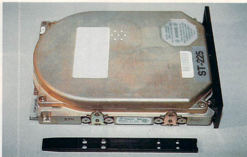
Most AT computers use plastic rails that you attach to the side of the drives. The drives slide on these rails into the drive cage.
