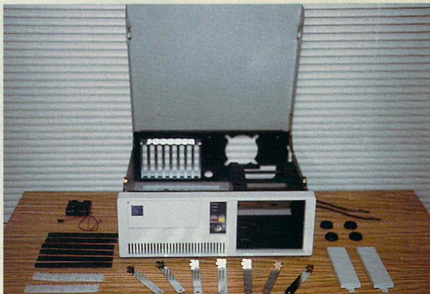
Begin by preparing the case. A "baby" AT case with a flip-open top is easier to work with than the standard slide-cover case.
