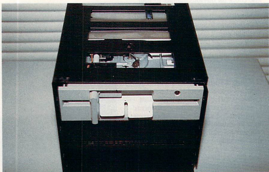
Once you've placed the drives in the cage, the entire assembly can be installed in the case.
