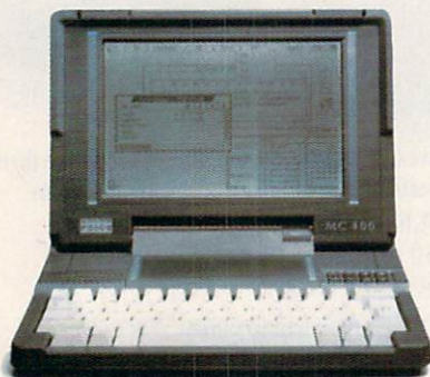
The Psion MC-400 accepts up to four solid-state disks at one time.
