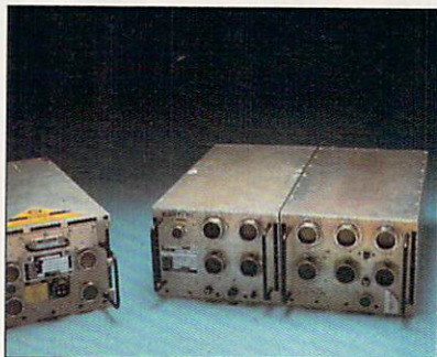
The AP-101S (left) uses only one box, operates three times faster, and is twice as reliable as its 18-year-old cousin, the AP-101 (right).
