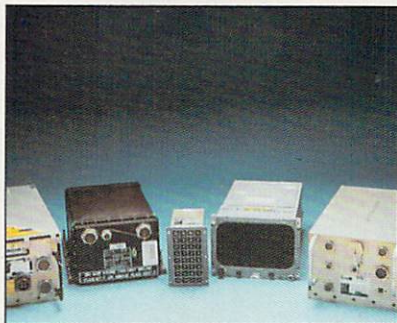
Left to right: AP-101S General Purpose Computer (GPC), Mass Memory Unit (MMU), Keyboard, Display Unit (DU), and Display Electronics Unit (DEU).
