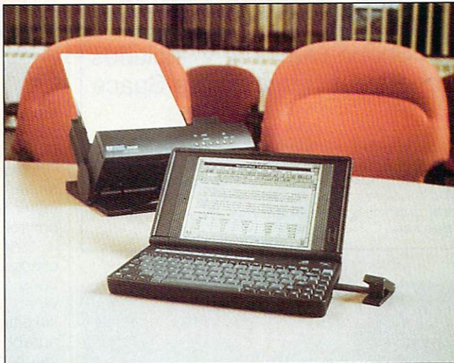
Hewlett-Packard's OmniBook 300 packs up to ten hours of battery power and Windows in ROM in a 2.9 pound package.
