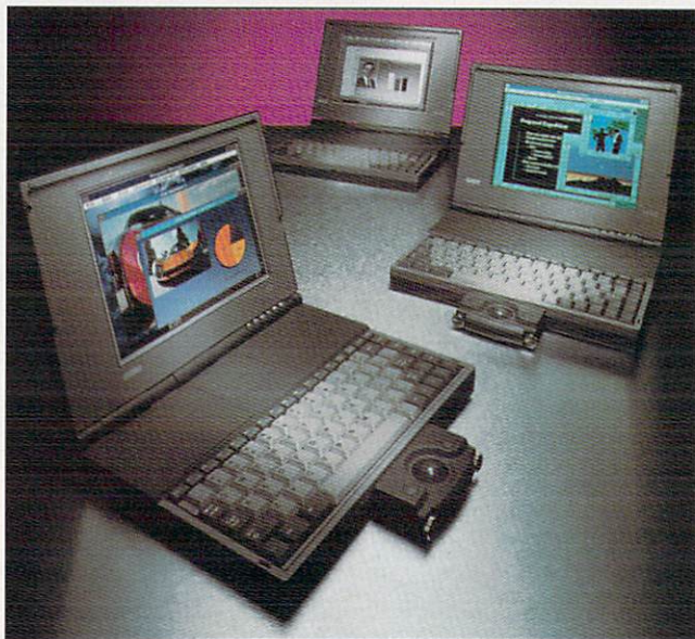
The NCR 3150 sports a fast 25-MHz 486SX processor, available active-matrix color, and a front-mounted trackball.
