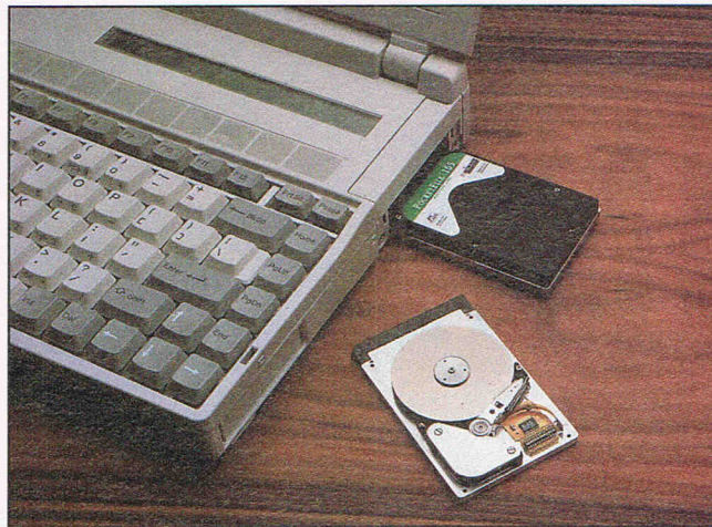
The PocketFile 85 PCMCIA card packs 85 megabytes of hard disk storage into a package the size of a thick credit card.
