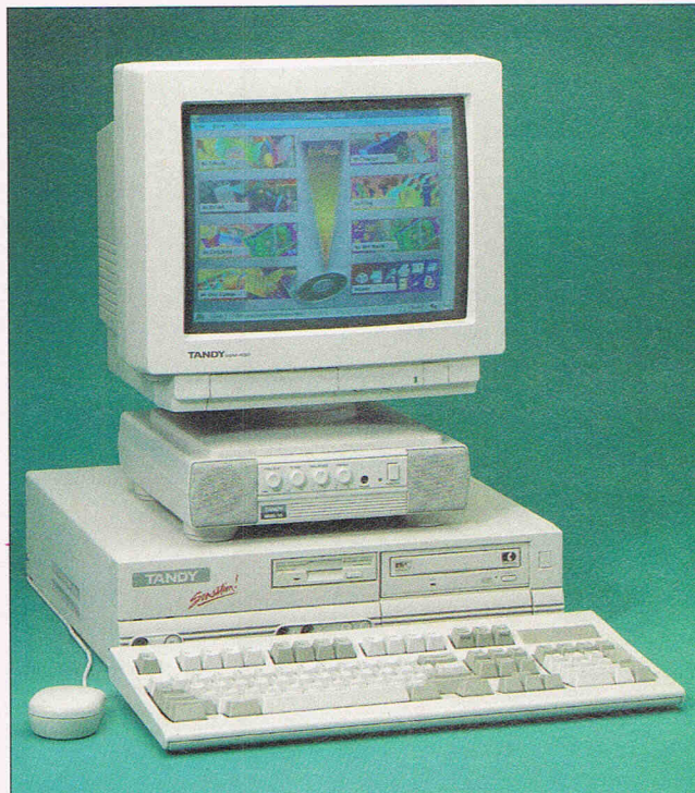
Tandy's 1994 Sensation sports a 16-bit sound card, double-speed CD-ROM drive, and voice-mail modem.
