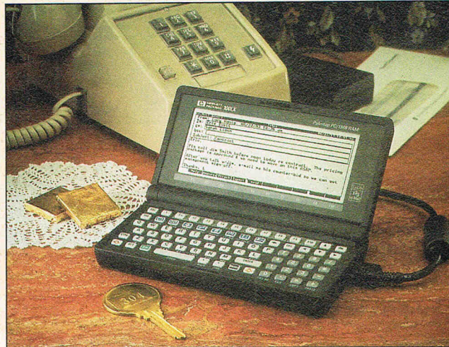
Hewlett-Packard's HP100LX palmtop computer offers a full 80- x 25-line display and the ability to run most DOS programs.
