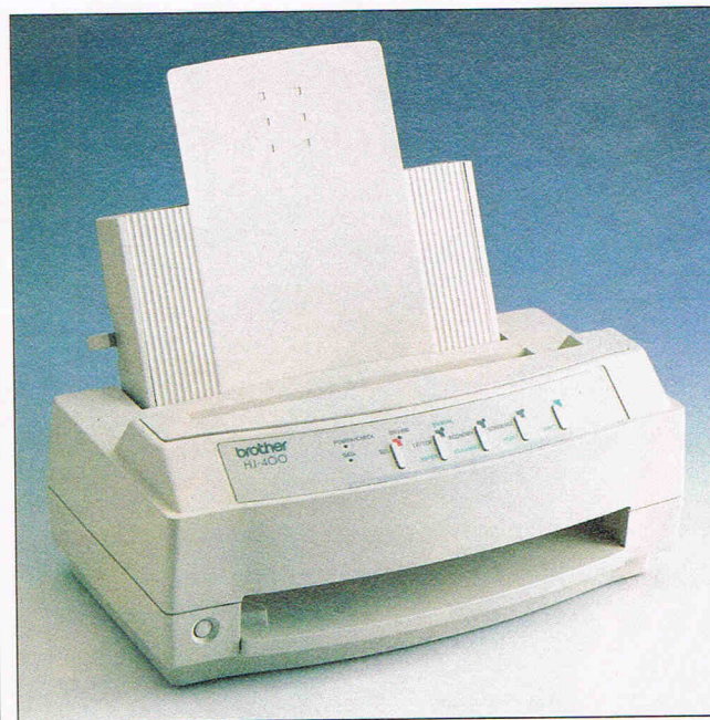
The Brother HJ-400 ink-jet printer sports a very small footprint, but it has an awkward sheet-feeder mechanism.
